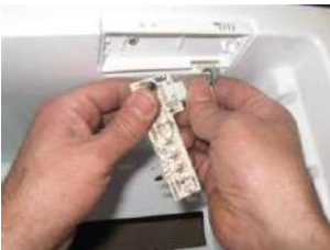
Remove the Led-Board and pull out the data cable.
